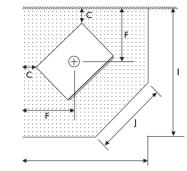
NOTE: The Hearth is not required to sit flush against the rear wall.
