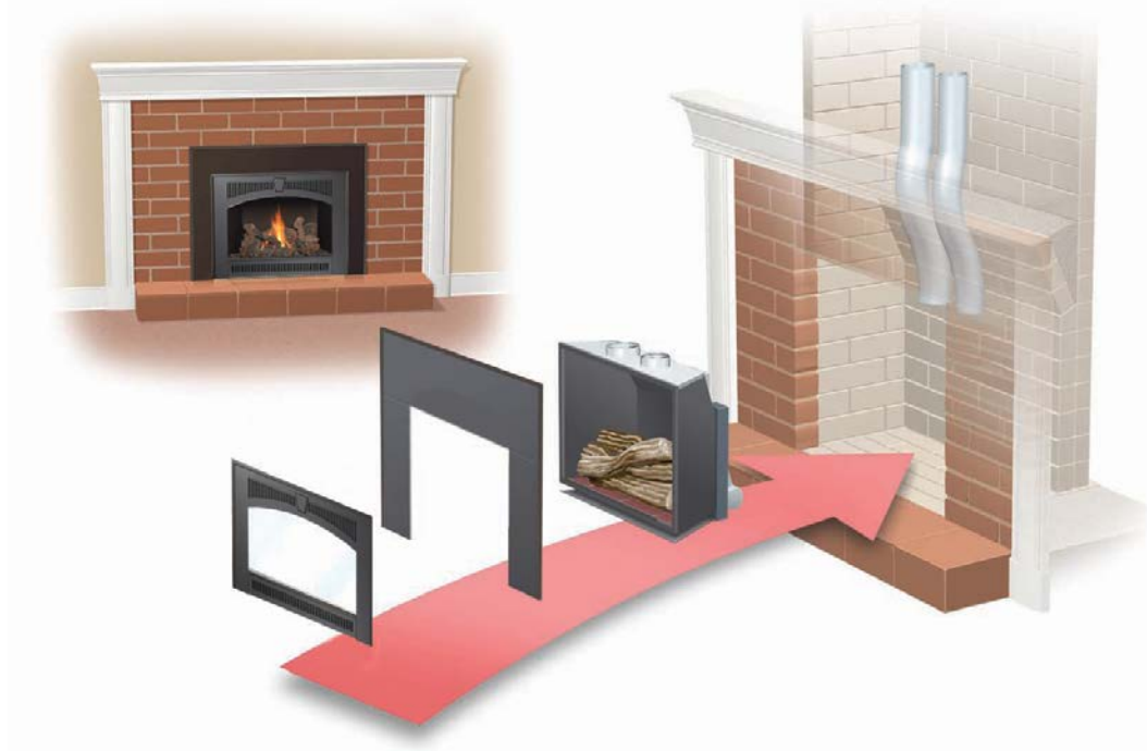
Flexible pipes are installed in your chimney and connect to a chimney termination seen left.
