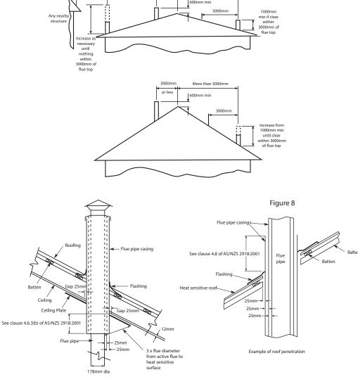
Example of sloped ceiling penetration
