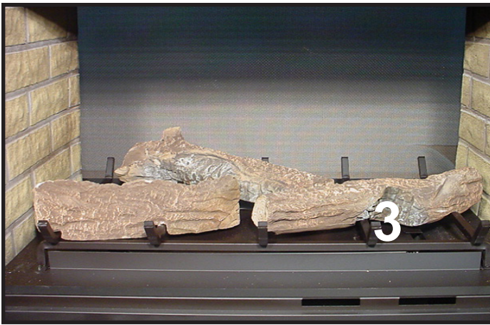
LOG #3 (SRV2068-702): Position log #3 across the third, fourth and fifth grate bars and push towards the rear against the grate tabs on bars three and five.
