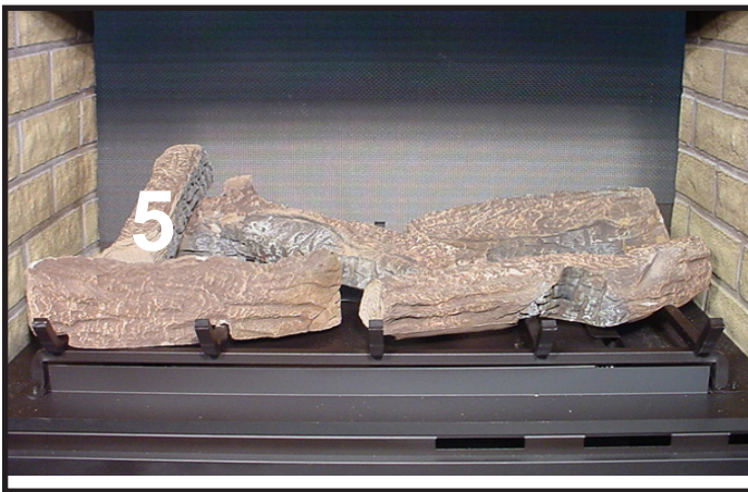
LOG #5 (SRV2068-703): Place log #5 on top of flat spot on log #1 and against the inside of log #2. Be careful not to reposition log #2 when placing this log.
