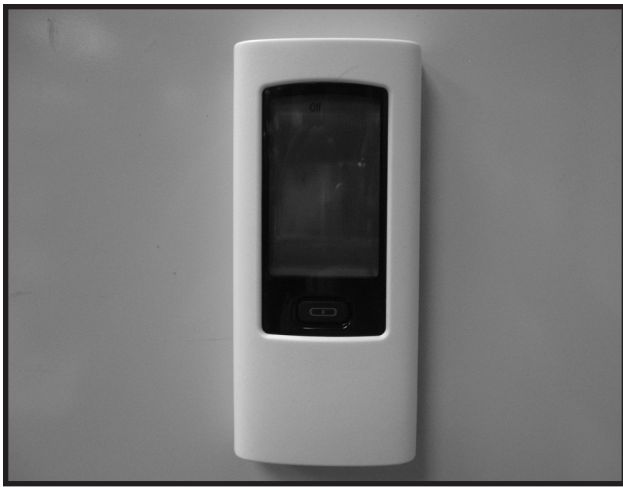
Figure 49. Mounting Remote Control Housing AUX300CE Module Installation
