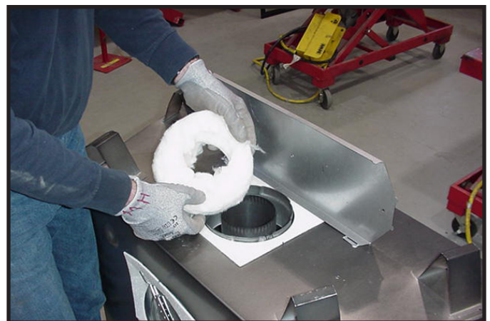
Figure 6.6 Remove the insulation from the outer vent pipe.
