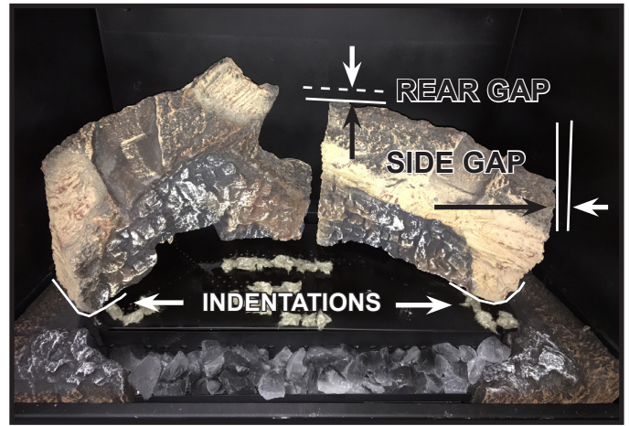
Figure 5. Rear Right Log Installed
