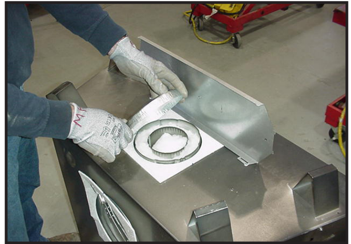
Figure 6.4 Remove the seal cap.
