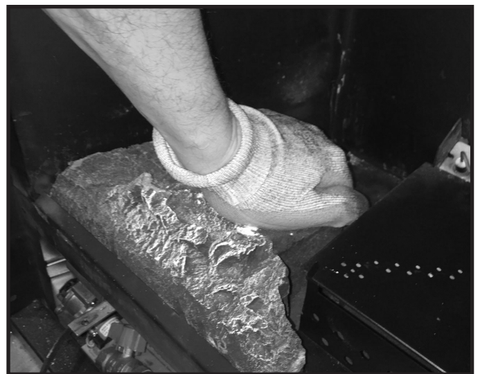
Figure 11.2 Press Left Hearth Firmly Into Place
