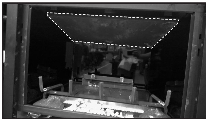
Figure 11.5 Install Top Refractory Panel
